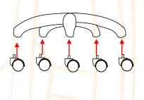
Step 2. Insert the cylinder into the pre-assembled Base.
