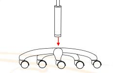
Step 3 . Place The Telescopic on top of the Cylinder (not on all models)
